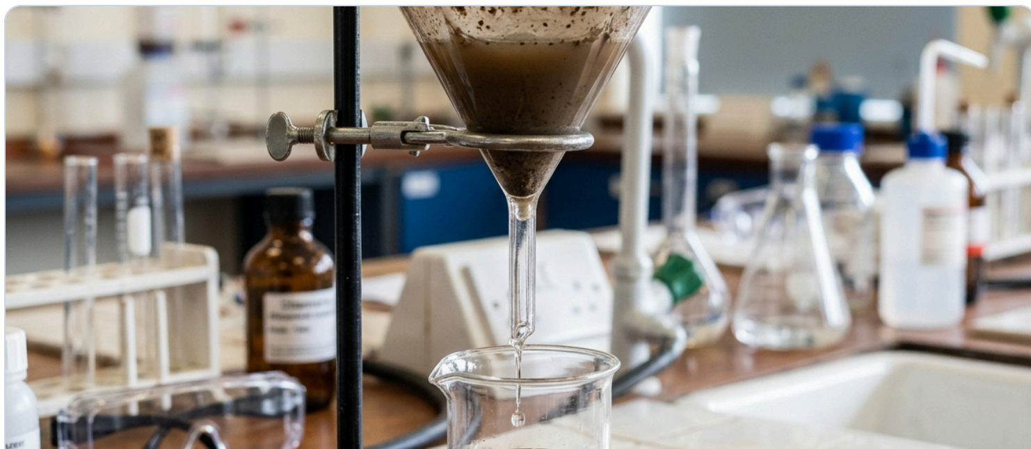
Figure 9.3: Filtration of Muddy Water (Coursebook Page 179) — Funnel lined with filter paper. The solid particles trapped on the filter paper are called residues , while the clear water dripping into the beaker is the filtrate .
