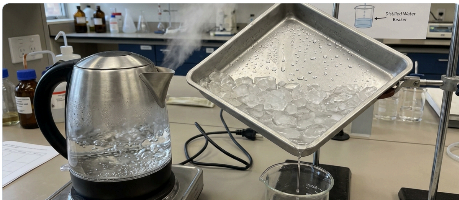
Figure 9.5: Water Distillation Method (Coursebook Page 181) — Muddy water boils in a kettle, steam hits a tilted cold metallic tray cooled by ice, and condenses into clean droplets of distillate water.
