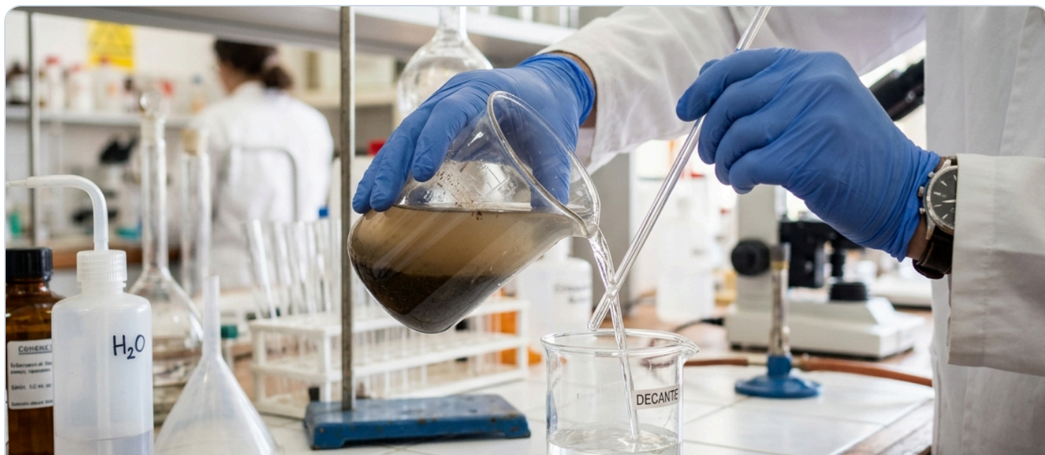
Figure 9.4: Decantation Process Using a Glass Rod (Coursebook Page 181) — Pouring off clean water along a glass stirring rod into another beaker, leaving settled mud and precipitate undisturbed at the bottom.
