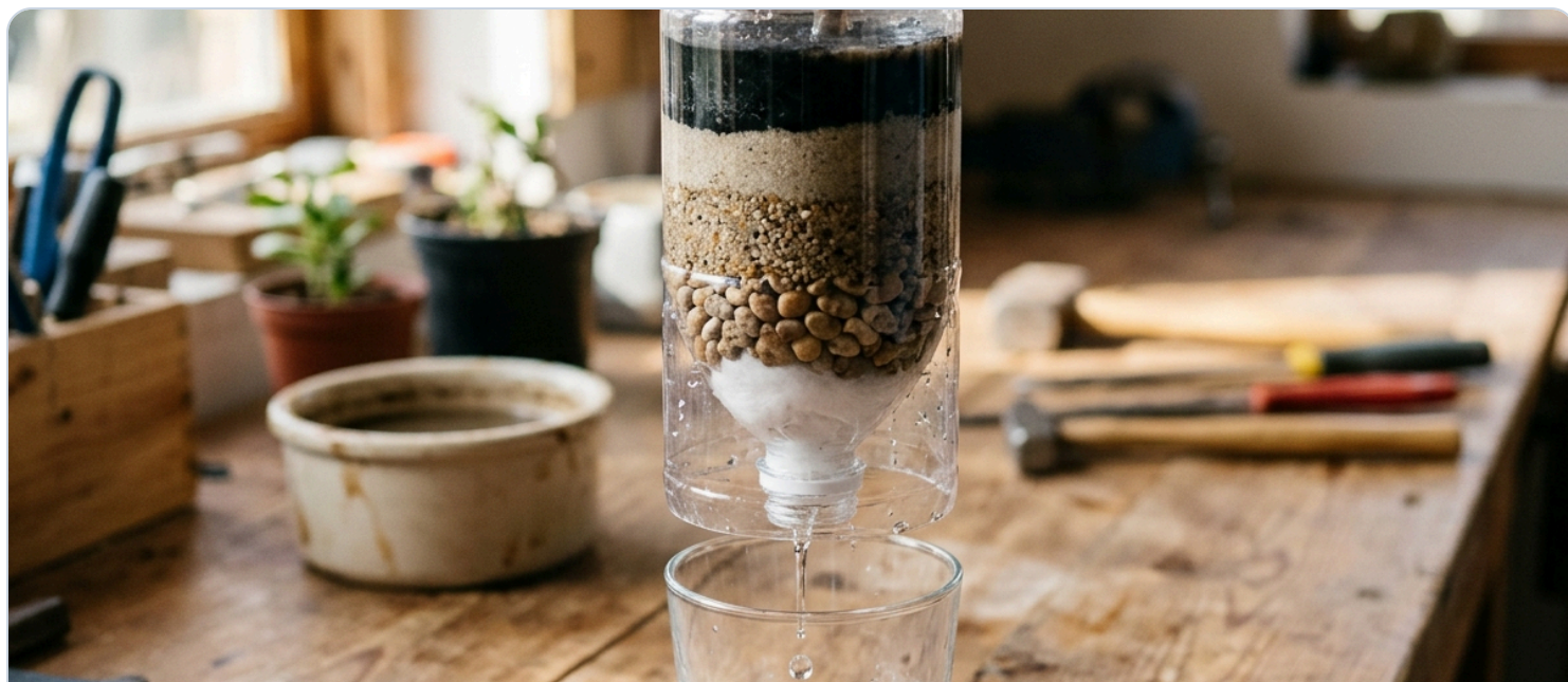
Figure 9.7: Simple Homemade Water Purifier Column (Coursebook Page 182) — Inverted plastic bottle showing stacked layers: dirty water → charcoal paste → fine sand → coarse sand → pebbles → cotton wool → clean water.
